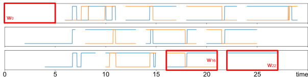
Figure 3: Binary local speaker segmentation. For each step of the 5s window w , only K_w \in \{0, 1, 2, 3\} speakers whose probability goes above \theta are kept.
