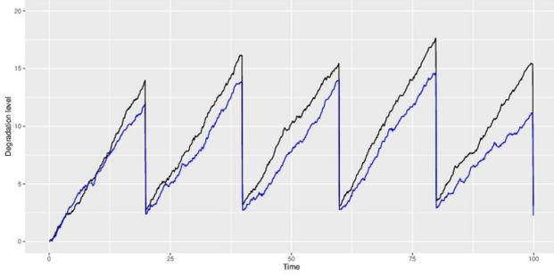
**Figure 1.** ARD( $\infty$ ) with repair efficiency parameter  $\rho = 0.9$ .
