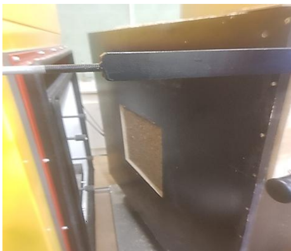
Figure. 12. S/BP wall insertion in the Thermo 3 device
