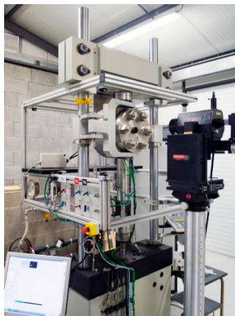
Fig. 1. Hycomat test bench used to perform in-situ FCGR tests.
