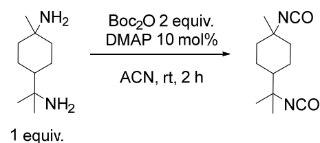
Scheme 2. Synthesis of PMDI from PMDA under phosgene-free conditions.
