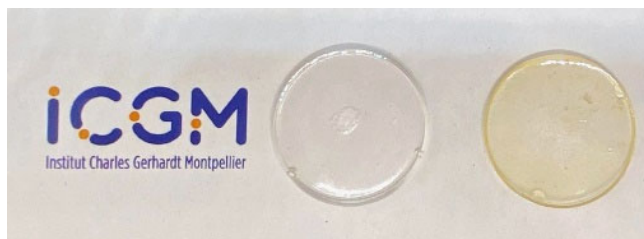
Figure 7. Photograph of IPDI-based thermoset (left) and PMDI-based thermoset (right).
