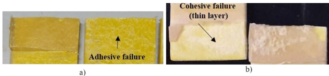
Fig. 9. Representative fracture surfaces of E LTX samples (a) untreated and (b) treated with UA.
