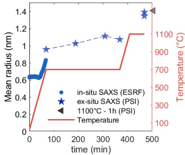
Fig. 3: Evolution of the mean radius of nano-oxides on CP specimens
