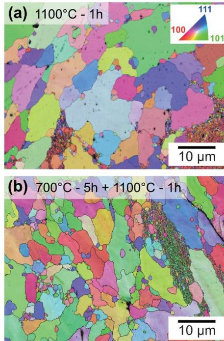
Fig. 1: EBSD orientation mapping of the final stage of the thermal treatment without 700 °C plateau (a), and with 700 °C plateau (b), displaying similar microstructures.
