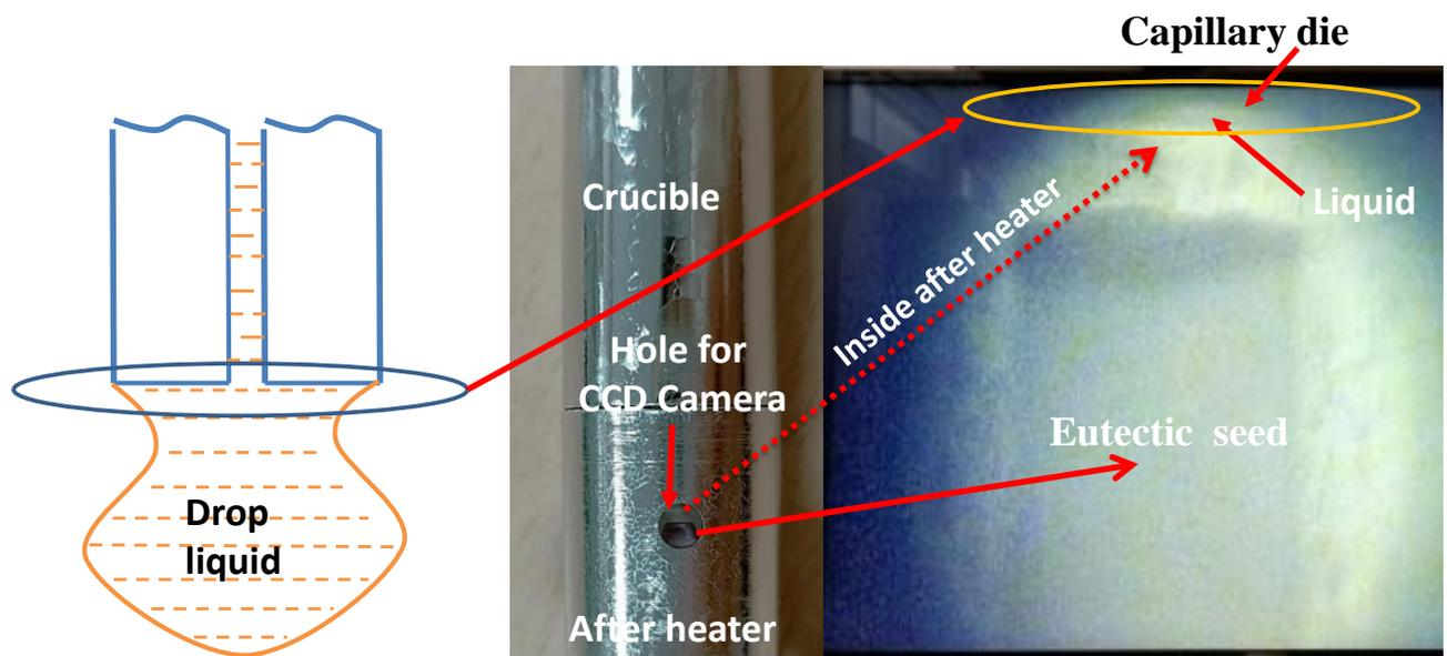
Fig. 1. Schematic illustration of the drop at the bottom of the capillary die (left), CCD camera vision of the growth initiation through the crucible and after heater (right)
