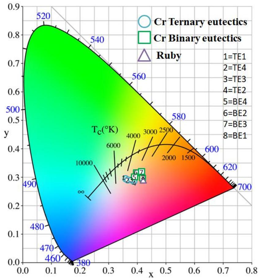
Fig. 3. CIE-1931 chromaticity diagram as a function of Cr concentration in the binary and the ternary eutectic
