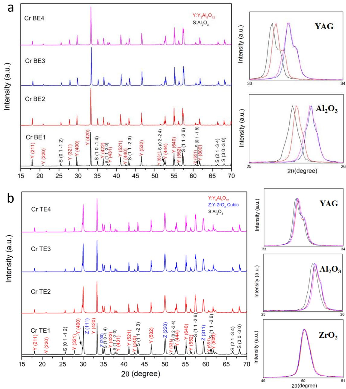
Fig. 4. X-ray diffraction evolution as a function of Cr dopant concentration, (a) Al<sub>2</sub>O<sub>3</sub>-YAG binary system and (b) Al<sub>2</sub>O<sub>3</sub>-YAG-ZrO<sub>2</sub> ternary system.
