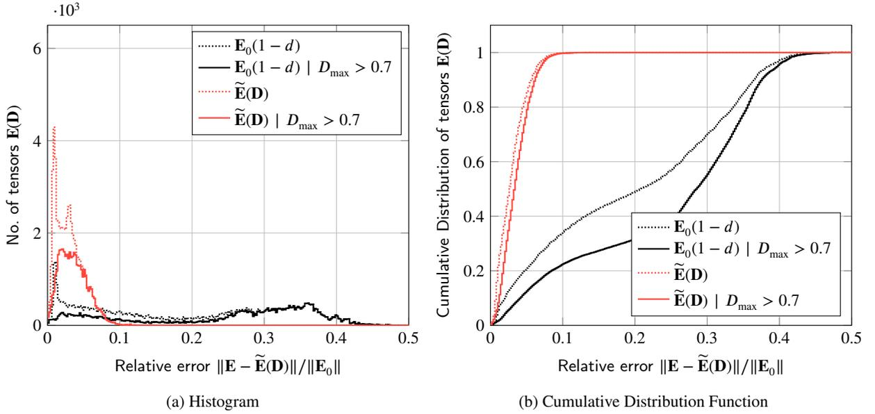
**Figure 17:** Histograms and Cumulative Distribution Functions of total error for large values of damage. The histogram and cumulative distribution of total error over the elasticity tensors in the dataset is also reproduced.
