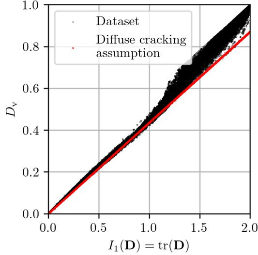
**Figure 9:** Check of the assumption of total symmetry of the stiffness loss tensor: the dots in black correspond to the value in the dataset and the red dots correspond to the  $D_v$  computed via Equation 41
