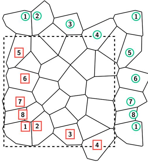
**Figure 3:** Periodic beam-particle mesh where the red boxed particles are guiding particles and green circled ones are guided particles. Guided particles have the same number as their guiding particle.
