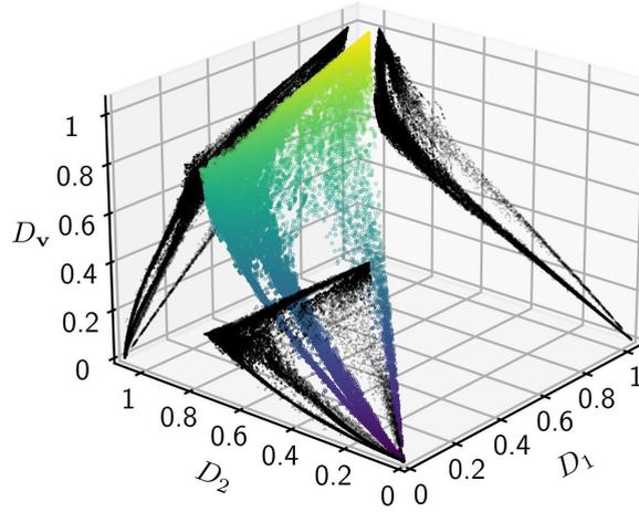
**Figure 8:** Damage  $D_v$  as a function of the eigenvalues  $D_1$  and  $D_2$  ( $D_2 > D_1$ ) of the damage variable  $\mathbf{D}$  over the dataset. Each colored point is the value of  $D_v$  for an elasticity tensor of the dataset. The black dots are the projections of the data points onto the planes  $(D_1, D_v)$ ,  $(D_2, D_v)$  and  $(D_1, D_2)$ .
