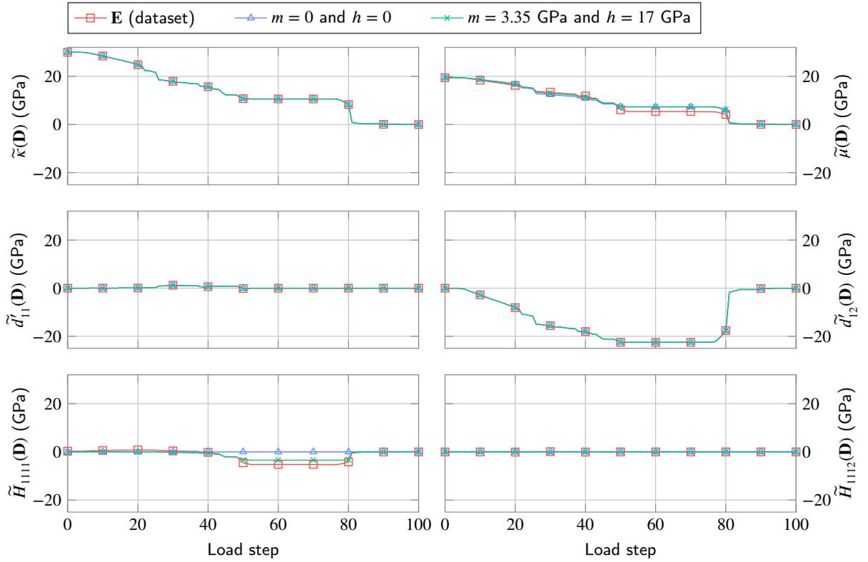
**Figure 18:** Comparison of the evolutions of elasticity tensors obtained via the two modelings ( $m = h = 0$  in blue, and  $m = 3.35$  GPa,  $h = 17$  GPa in green) with the reference data ( $\mathbf{E}$ , in red) during a shear→tension loading.
