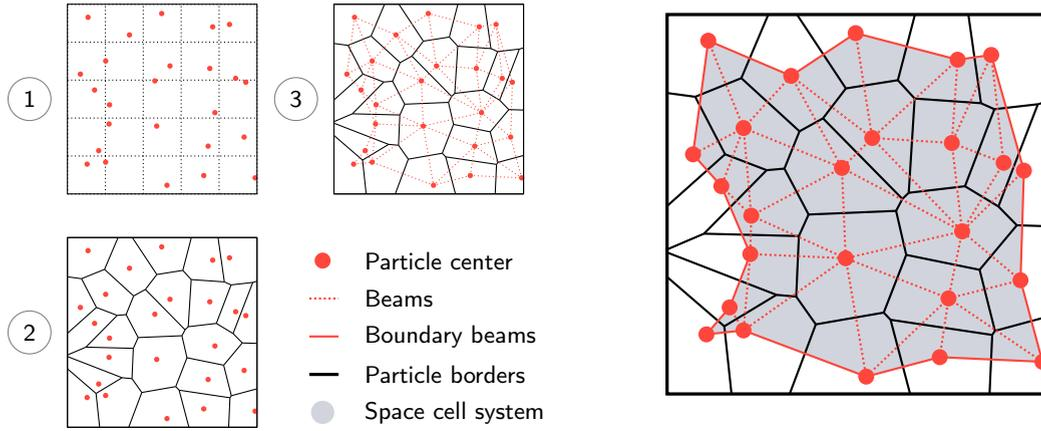
**Figure 1:** Representation of the mesh of the beam-particle model. (1) is the positioning of the particle centers in the grid. (2) is the generation of the particle border by the Voronoi tessellation of the particle centers. (3) adds the beam network based on the Delaunay triangulation of the particle centers.
