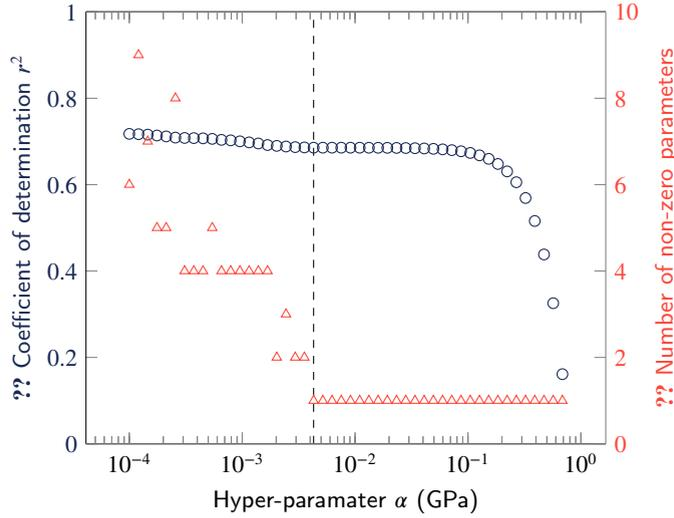
**Figure 12:** Illustration of the compromise between the precision and the number of non-zero parameters in the constrained LASSO regression. The dashed line shows the best compromise for us ( $\alpha = 0.0043$  GPa).
