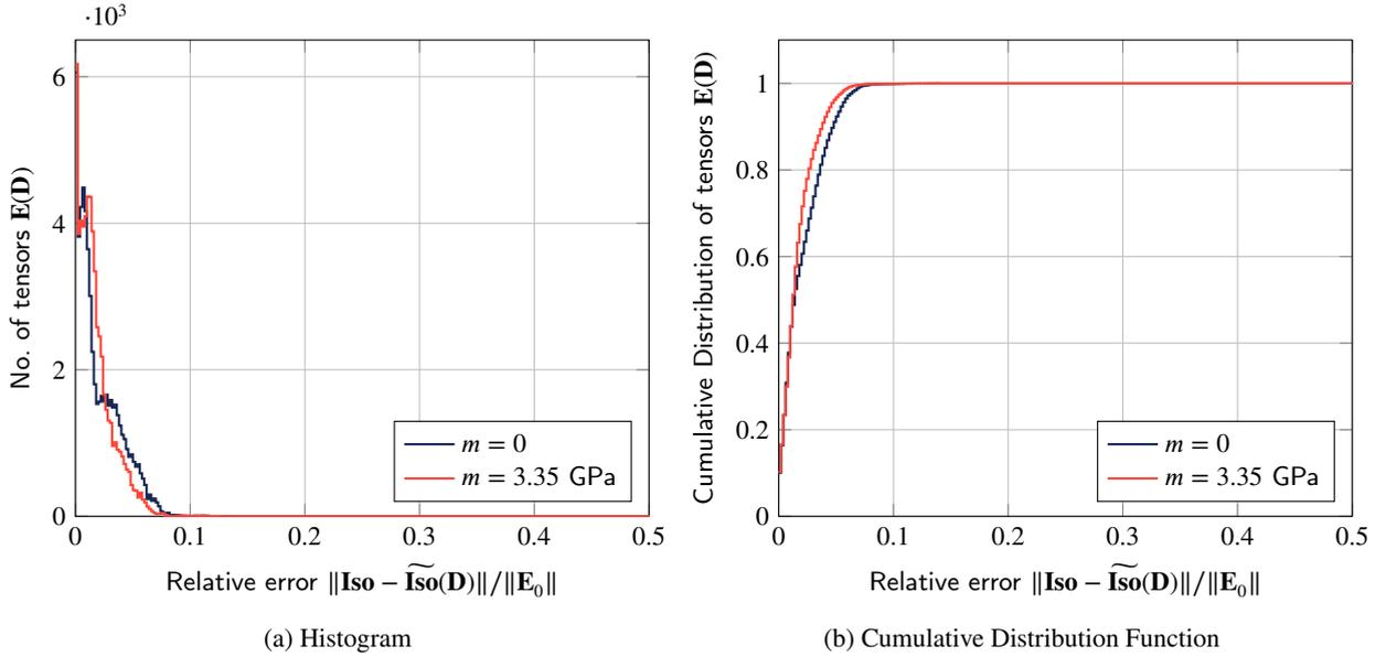
**Figure 14:** Histograms and Cumulative Distribution Functions of the relative error on the isotropic part over the dataset for both values of  $m$  (results independent from the harmonic prefactor  $h$ ).
