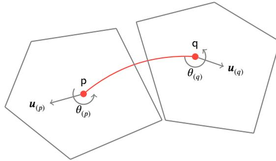
**Figure 2:** Representation of a beam and notations
