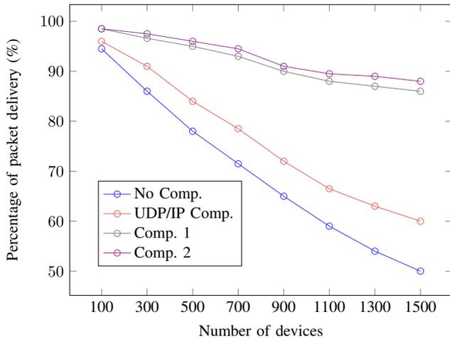
Fig. 6. Percentage of packet delivery with respect to the number of devices for different compression types.
