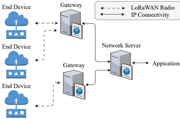
Fig. 1. LoRaWAN Architecture [7].
