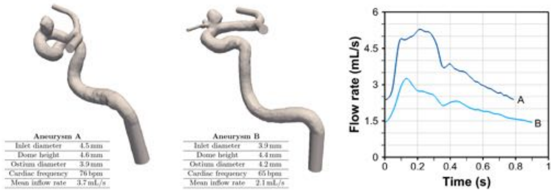
Figure 1. Patient-specific geometries and datasets for the two ICA aneurysms investigated in this study. The rightmost plot provides one period of the patient-specific inflow pulses used for the CFD simulations. The range of Reynolds numbers in the parent vessel (based on the inlet diameter, inlet velocity and infinite-shear rate viscosity) is 220-490 for patient A, and 160-370 for patient B (resp. at diastole and systole).
