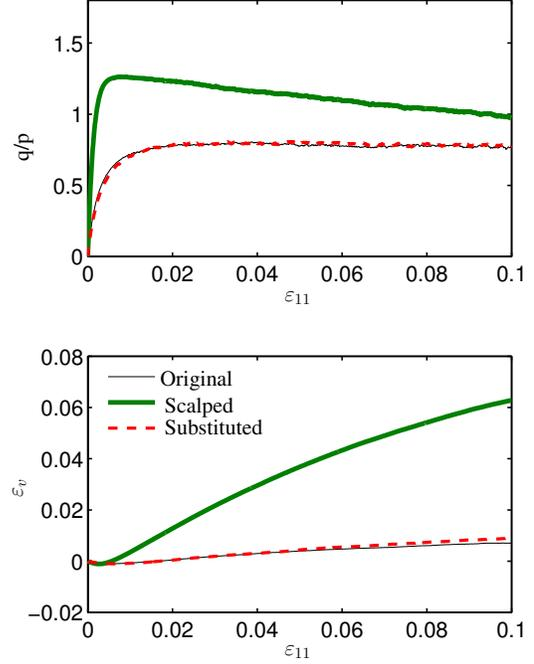
**Fig. 8:** Stress ratio  $q/p$  and volumetric strain  $\varepsilon_v$  versus axial strain  $\varepsilon_{11}$  for the original sample with  $f_f = 60\%$  and its scalped and substituted samples.  $e = 0.49$  is controlled for all the samples.
