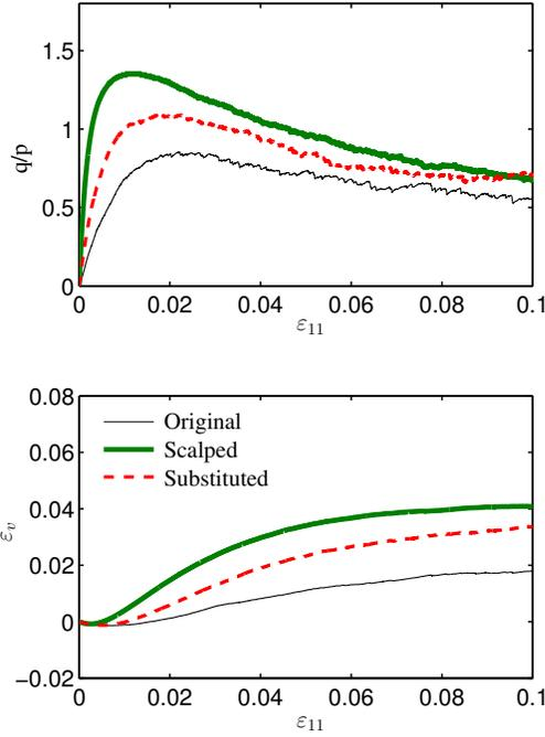
**Fig. 7:** Stress ratio  $q/p$  and volumetric strain  $\varepsilon_v$  versus axial strain  $\varepsilon_{11}$  for original samples with  $f_f = 30\%$  and its scalped and substituted samples.  $e = 0.36$  is controlled for all the samples.
