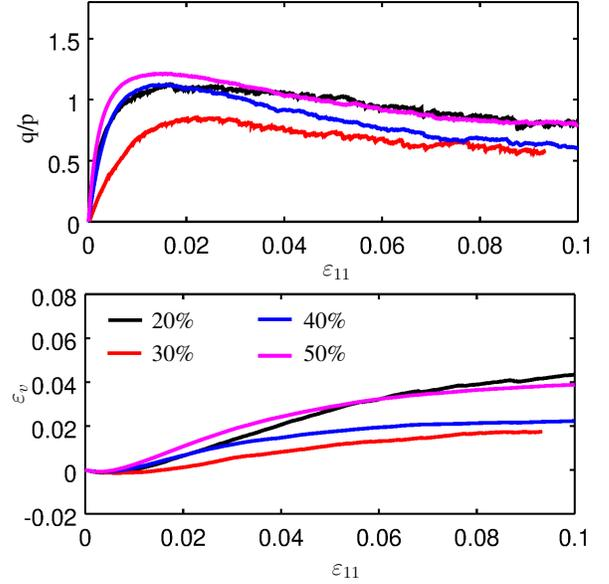
**Fig. 10:** Stress ratio  $q/p$  and volumetric strain  $\varepsilon_v$  versus axial strain  $\varepsilon_{11}$  for different fine contents  $f_f$  when the global fine content  $e$  is controlled to be almost the same.
