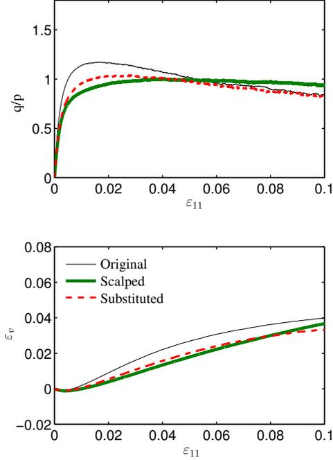
**Fig. 5:** Stress ratio  $q/p$  and volumetric strain  $\varepsilon_v$  versus axial strain  $\varepsilon_{11}$  for original sample with  $f_f = 60\%$  and for the scalped and substituted samples.  $D_R = 50\%$  is controlled for all the samples.
