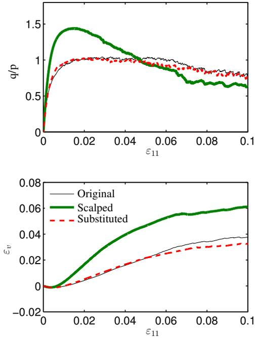
**Fig. 3:** Stress ratio  $q/p$  and volumetric strain  $\varepsilon_v$  versus axial strain  $\varepsilon_{11}$  for original sample with  $f_f = 20\%$  and for the scalped and substituted samples.  $D_R = 50\%$  is controlled for all the samples.
