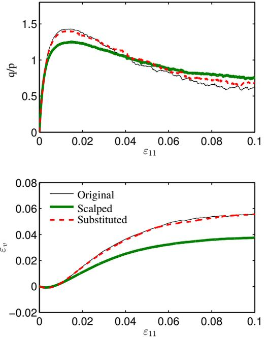
**Fig. 4:** Stress ratio  $q/p$  and volumetric strain  $\varepsilon_v$  versus axial strain  $\varepsilon_{11}$  for original samples with  $f_f = 30\%$  and for the scalped and substituted samples.  $D_R = 50\%$  is controlled for all the samples.
