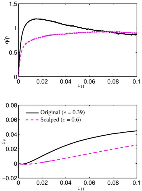
**Fig. 2:** Stress ratio  $q/p$  and volumetric strain  $\epsilon_v$  versus axial strain  $\epsilon_{11}$  for the original sample with  $f_f = 60\%$  and the scalped one. The void ratio  $e_{\text{retained}}$  of the retained fraction is controlled.
