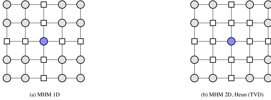
Figure 1: Sketch of the spatial stencils of the finite volume schemes considered in this work. \bullet : node where the fluxes are computed, \square : points considered in the computation of the fluxes, \circ : points not considered.
