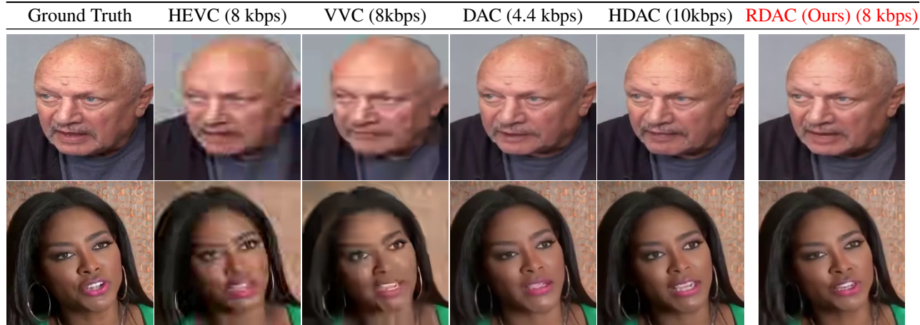
Fig. 2: Visual Comparison of coding results. A qualitative comparison of our proposed coding framework shows significant quality improvement over HEVC and VVC at low bitrates. We observe fewer smoothing and blocking artifacts as well as better color and style preservation in the reconstructed frames with our framework.
