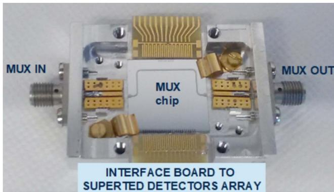
**Figure 20.** Picture of the iKID readout scheme prototype with two different materials. The matrix of thirteen resonators is in the center. Only the readout line is clearly visible: it is the horizontal line. The bottom PCB-board is connected to the resonators and to the cables.
