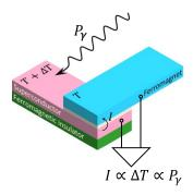
**Figure 2.** Schematic idea for biasless detection based on thermoelectricity. Absorbed light with power  $P_{\gamma}$  heats up one part of the heterostructure, creating a temperature difference  $\Delta T$ , which results in a thermoelectric current  $I = \alpha \Delta T/T \propto P_{\gamma}$ .
