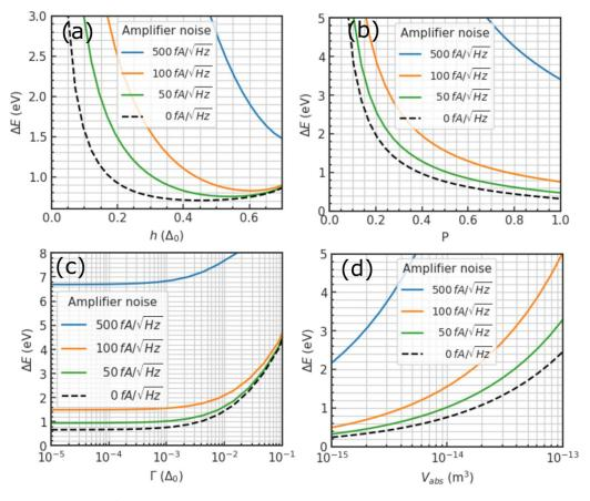
Figure 13. Total energy resolution  $\Delta E$  (including amplifier noise) plotted as a function of (a) exchange field h, (b) polarization P, (c) broadening parameter  $\Gamma$  and (d) absorber volume  $V_{abs}$ . The three colored lines demonstrate  $\Delta E$  with three different current read-out noise levels, and the black dashed line demonstrates the intrinsic resolution. Panel (d) is computed with materials parameters for an Sn absorber.
