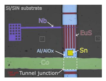
**Figure 15.** Fake-color optical micrograph of a SFTED calorimeter, in which the material compositions are illustrated with different colors. A superconductor–ferromagnet heterojunction area is marked with the white dashed line, consisting of layers of  $Si/SiN/EuS/Al/AlO_x/Co$  from the bottom to the top. A Sn absorber is placed to the side of the junction, contacting directly the Al lead with  $AlO_x$  layer removed via chemical etching.
