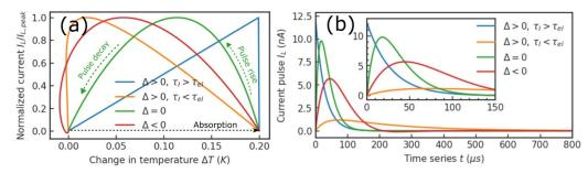
**Figure 14.** (a) Current-temperature pulse cycles under different operational conditions, denoted by the color of the lines. (b) Signal current pulse under different operational conditions corresponding to panel (a).
