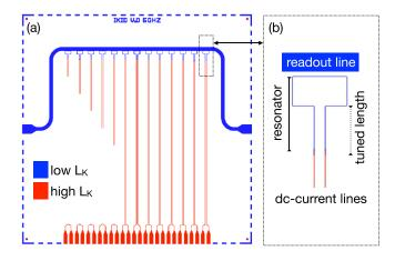
**Figure 19.** Design of the iKID readout scheme with two different materials design (a) Resonators (in blue) are to connect to the detectors (not shown) via the dc-current lines (in red). The blue horizontal line is a readout line to monitor the resonance frequencies. (b) Zoom on a resonator.
