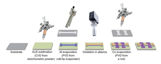
Figure 6. Schematic representation of the different steps involved in the hybrid heterostructure growth.
