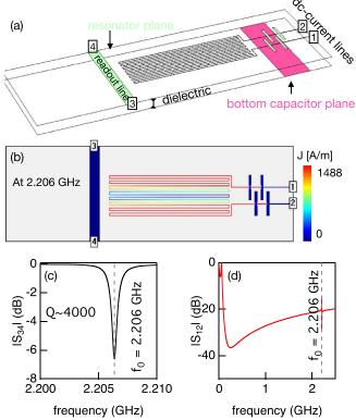
**Figure 21.** Electromagnetic simulation of a promising configuration of iKID based on 3D lumped-element capacitance. (a) 3D-model. The dielectric is a 30 nm thick alumina. The metal, green and pink, is aluminum. (b) Current distribution at the resonance. (c) Electrical response of the KID. The quality factor of the resonance is of about  $4 \cdot 10^3$ . (d) Electrical response of the DC-lines. The DC-lines are low pass filters.
