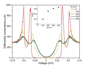
**Figure 8.** Differential conductance as a function of in-plane external magnetic field for sample S1-b. Subgap states and delta vary with B. The inset shows the field dependence of the zero bias conductance  $G_0(B)$  normalized respect to the normal state conductance  $G_N$ .
