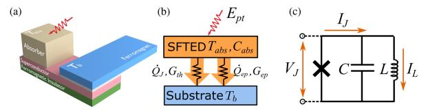
Figure 11. Schematic of a (a) superconductor–ferromagnetic thermoelectric detector (SFTED). (b) and (c) are the thermal model and the electrical circuit of the SFTED.
