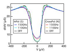
**Figure 17.** Conductance-voltage characteristics of the SFTED junction shown in figure 16 under different illumination conditions. In particular, varying the direction of the polarisation and the frequency of the millimetre-wave source.  $H = 20 \, \text{mT}$  along the direction of the superconductor (S) and  $T = 120 \, \text{mK}$ .
