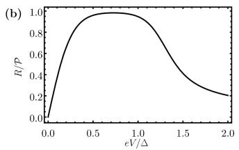
**Figure 5.** (a) I(V) curve of a N/FI/S junction for different values of the polarization  $\mathcal{P}$ . (b) Rectification coefficient  $R = I_{\rm sym}/I_{\rm asym}$ . Parameters used in the plots:  $h = 0.3\Delta$ ,  $k_BT_N = k_BT_S = 0.1\Delta$ ,  $\Gamma = 10^{-3}\Delta$ .
