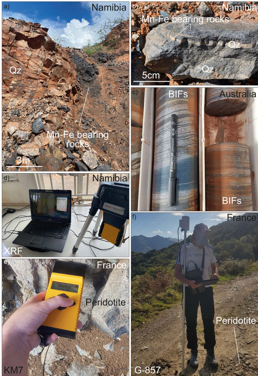
Fig. 12. Images showing different outcrops, samples, and various in situ analyses. (a, b) Mn-Fe bearing rocks in Namibia. (c) BIF core from Australia. (d) Portable XRF instrument for in situ major element analysis. (e, f) Kappmeters KM7 and G-857 for magnetic susceptibility measurements. See Appendix B for coordinates.
