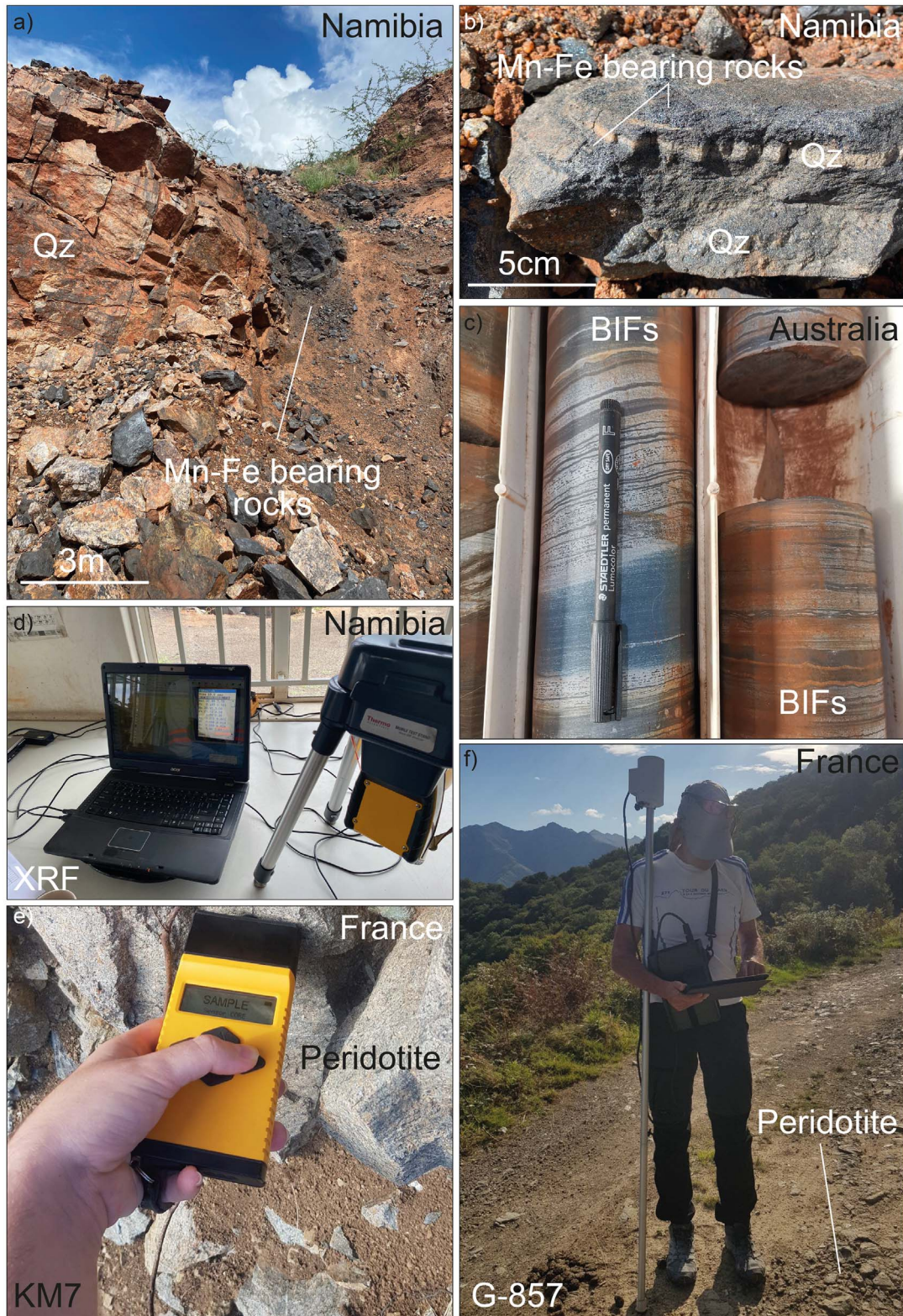
Fig. 12. Images showing different outcrops, samples, and various in situ analyses. (a, b) Mn-Fe bearing rocks in Namibia. (c) BIF core from Australia. (d) Portable XRF instrument for in situ major element analysis. (e, f) Kappmeters KM7 and G-857 for magnetic susceptibility measurements. See Appendix B for coordinates.
