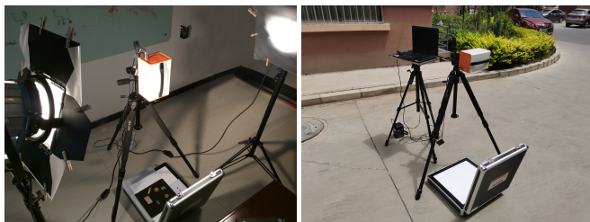
Fig. 8. Indoor (left) and outdoor (right) experimental setups for collecting real data.
