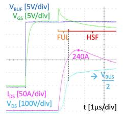
Fig. 9: Highlight of the high-side FUL-HSF sequence subsequently to a low-side HSF.
