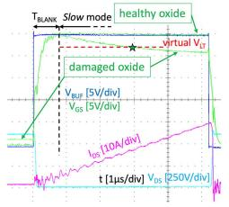
Fig. 13: Experimental highlight of healthy and damaged oxides' impact on  $V_{GS}$  ON-state waveform. The DUT with a damaged oxide underwent consequent thermomechanical stress due to several short-circuit and overload tests before the appearance of a significant gate-oxide leakage current.
