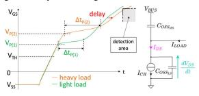
Fig. 10: Simplified illustration of the impact of the load current on  $V_{GS}$  dynamics, equivalent schematic.
