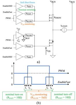
Fig. 1: a) Proposed parallel 2-channel Fast-lane and Slowlane SiC MOSFET gate-driver, b) Enable and PWM control signals ( $t_1 = t_3 = 50$ ns,  $t_2 = t_4 = 830$ ns).
