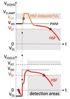
Fig. 8: Simplified illustration of the impact of a low-side HSF short on LS and HS gate voltage waveforms.
