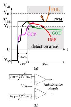
Fig. 4: a) Illustration of different fault signatures on  $V_{\rm GS}$  (T\_{\rm BLANK} = 830ns), b) double threshold fault detection principle.
