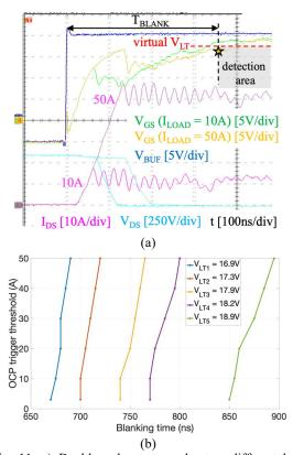
Fig. 11: a) Double pulse tests under two different load current levels  $I_{LOAD}$  [10A; 50A] - highlight of the OCP principle of detection (detection inhibited), b) experimental parametric results on the impact of the blanking time on the OCP trigger threshold for different  $V_{LT}$  ( $R_{FAST} = 47\Omega$ ,  $V_{DD} = 20V$ ,  $V_{SS} = -5V$ ,  $V_{BUS} = 600V$ ).
