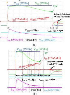
Fig. 3: HSF operation with safe FTO mode illustrations,  $V_{DD} = 20V$ ,  $V_{SS} = -5V$ , a) traditional single-channel gatedriver (R<sub>GATE</sub> = 270 $\Omega$ ,  $V_{DS} = 333V$ ), b) dual-channel Fast/Slow gate-driver architecture for different pulse durations until the appearance of the FTO mode (R<sub>FAST</sub> = 47 $\Omega$ , R<sub>SLOW</sub> = 4.3k $\Omega$  at a high voltage of V<sub>DS</sub> = 600V).
