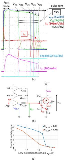
Fig. 5: a) Experimental HSF waveforms for different low detection thresholds  $V_{LT}$ , b) HSF equivalent schematic, c) parametric protection delay measured between the faulty turn-on and the activation of the SSD signal.
