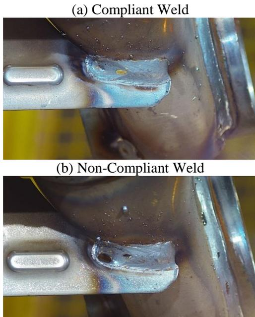
**Figure 6:** Examples of welds
