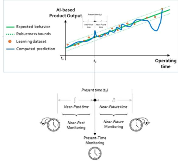
**Figure 3:** Principle of the multi-timescale online monitoring
