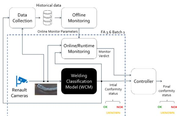
**Figure 7:** Online Monitoring of the Welding Classification Model
