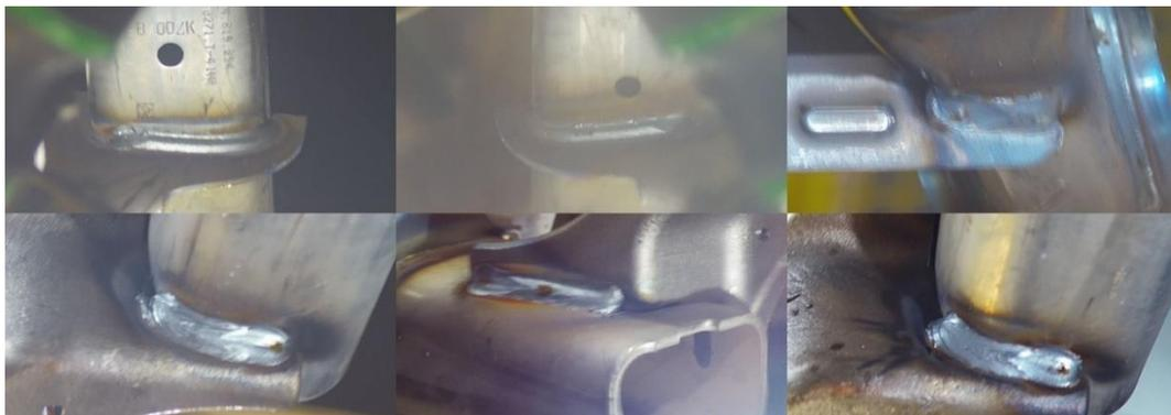
**Figure 10:** Blur Anomaly Detection on the Welding Use Case based on PTM monitoring
