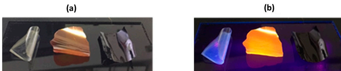
Figure 2. Thin films of polymers P1, P2 and P3 under (a) natural light and (b) UV-365 nm irradiation.
