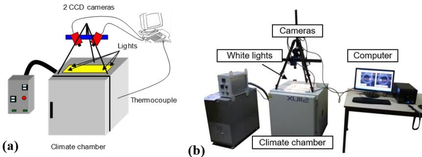
**Figure 2:** (a) Outline and (b) photo of the experimental set up.
