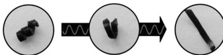
Figure 1. Deformed magnetic shape memory polymer, induction heated magnetic shape memory polymer in the process of recovering its memorized shape, recovered memorized shape [17].
