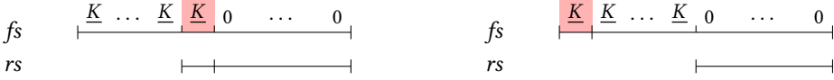
Fig. 22. Left: after snoc has inserted an element in the rear list. Right: before extract removes an element of the front stream. Highlighted in red: the thunk whose debit must be paid off.
