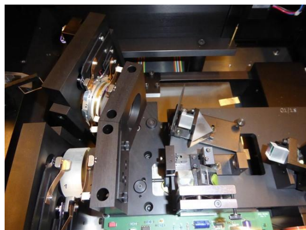
Figure 1. Photograph of the scanning 6-pass TFPI (TFP-2) used for the BLS measurement.
