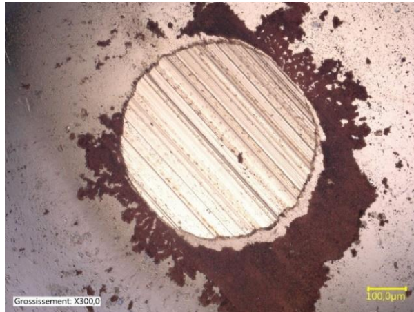
Figure S4 – Optical image of the wear track of a steel ball. Dark particles outside of the track are volatile particles.
