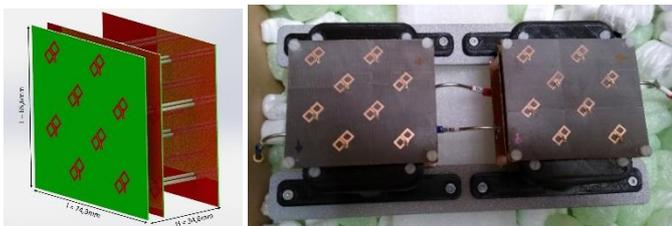
Fig. 4. X-Band antenna design and realisation
