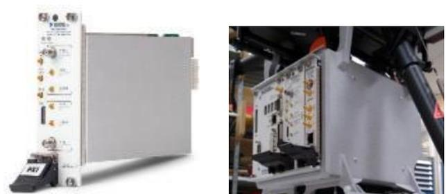
Fig. 2. PXIe generation and sampling board (left) and digital-core in 3D printed chassis (right)
