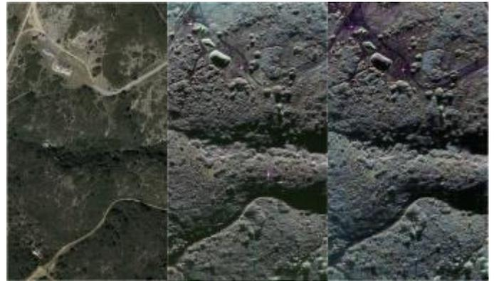
Fig. 10. GoogleEarth® (left), SAR-Light X-Band (middle), C-Band (right) imagery. Radar images are colour composition of quad pol (RGB = Hh, Hv, Vv) and high resolution (25 cm).
