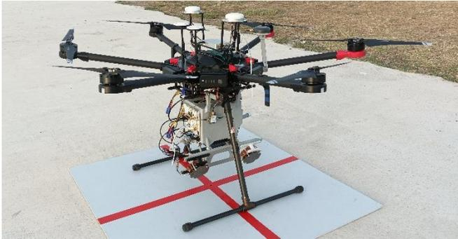
Fig. 8. C-Band SAR System on-board the DJI M600 platform
