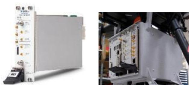
Fig. 2. PXIe generation and sampling board (left) and digital-core in 3D printed chassis (right)
