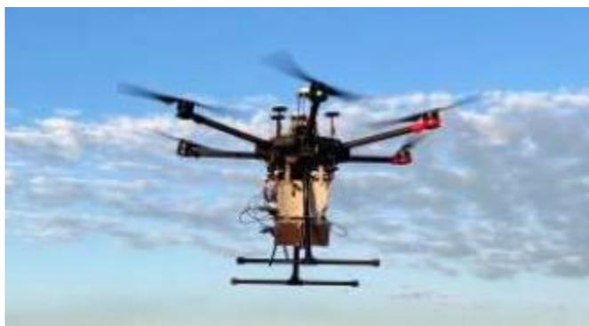
Fig. 1. SAR-Light platform based on DJI M600 UAV
