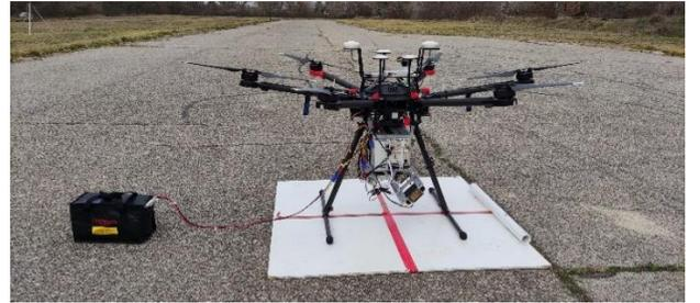
Fig. 6. X-Band SAR System on-board the DJI M600 platform
