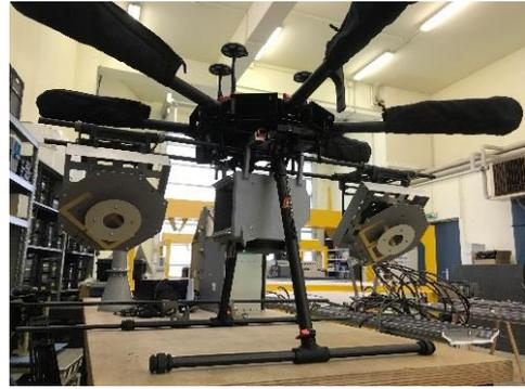
Fig. 9. UHF-Band SAR System on-board the DJI M600 platform
