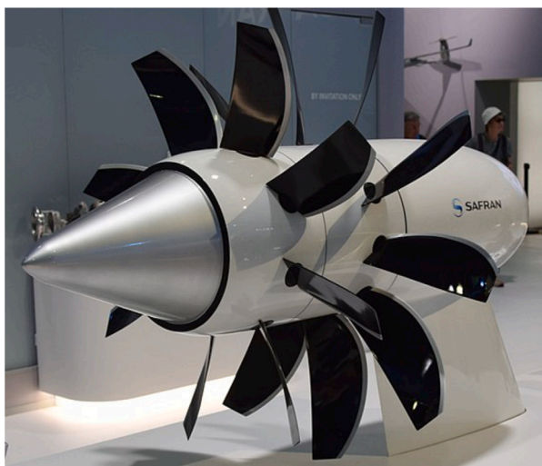
Fig. 10. Open rotor presented at the 2017 International Paris Air Show by Safran, after wikimedia commons .
