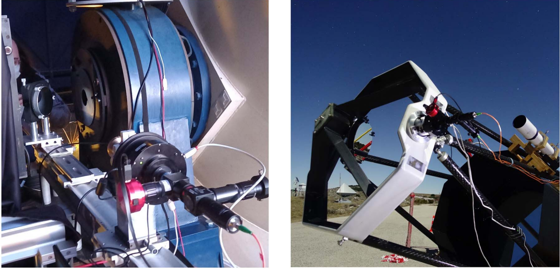
Figure 1. Photographs of the coupling assemblies mounted on the Nasmyth arm of the MEO telescope (left) and at the Newtonian focus of the TIM portable telescope (right).
