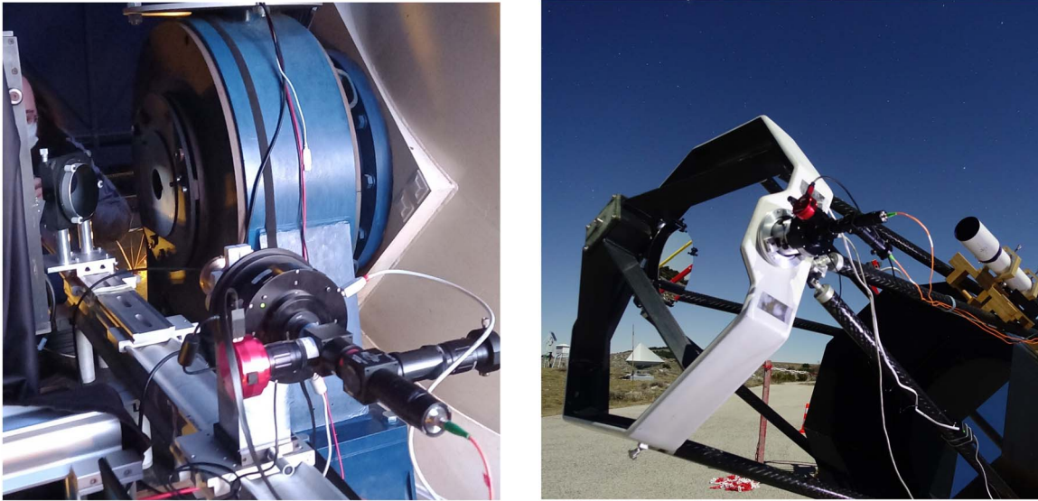
Figure 1. Photographs of the coupling assemblies mounted on the Nasmyth arm of the M&O telescope (left) and at the Newtonian focus of the TIM portable telescope (right).
