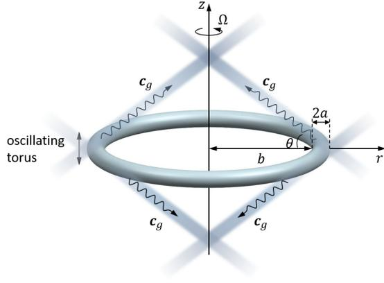
Figure 1. Schematic drawing of the oscillating torus and the focusing effect of the resulting inertial waves, where  $a$  is the radius of the tube and  $b$  the major radius of the torus with  $a \ll b$ ,  $\Omega$  is the constant angular velocity of the rotating flow.  $c_g$  denotes the group velocity, at which the wave energy propagates, and  $\theta$  is the propagation angle.
