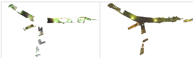
Figure 2. Horizontal section of underground galleries (1m wide) recorded by TLS (left: gaps due to the use of hybrid scanner as Trimble GX, and right: better coverage with the Leica C10 panorama scanner)
