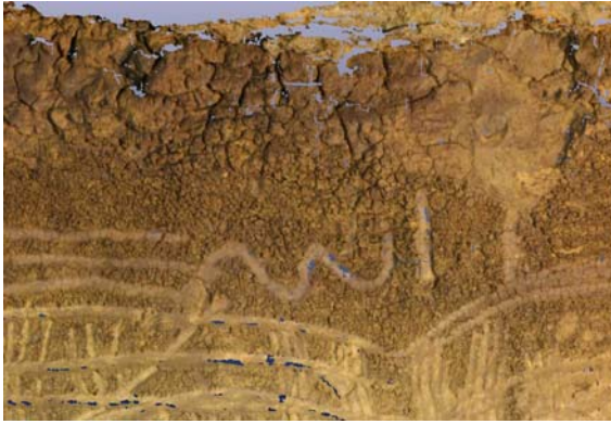
Figure 6. 3D textured raw model obtained by dense stereo matching from two panorama standpoints in front of the clay panel (the distance to object is 5m, focal length 85mm, pixel size in the object is less than 0,5mm, base/distance ratio is 0,4).
