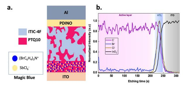
Figure 4: a) Schematic representation of the obtained architecture of the cell. b) ToF-SIMS measurements of the HTL and active layer stack deposited on ITO.
