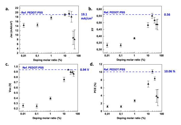
Figure 5: Solar cell parameters as a function of doping concentration in the PTQ10 interlayer. a) Short-circuit current density Jsc b) fill factor FF c) open-circuit voltage  $V_{oc}$  and d) power conversion efficiency PCE – blue mark is a guideline for the eye representing the reference PEDOT:PSS based solar cells.
