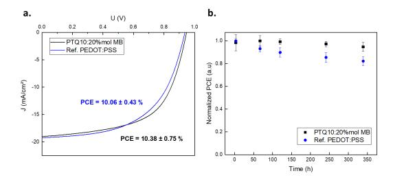
Figure 6: a) J-V curve of best device compared with Ref. PEDOT:PSS device. b) Device stability under inert atmosphere
