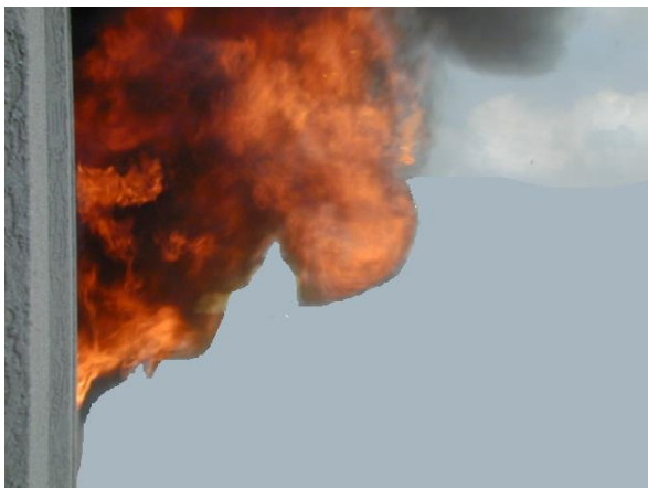
Figure 8. Ejected façade fire from compartment window due to the ventilation
