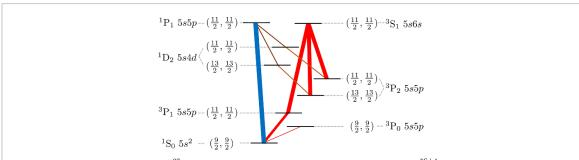
**Figure 7.** The energy diagram of the <sup>87</sup>Sr atom. Each state is labeled by both its electronic state  $^{2S+1}L_J$  and its hyperfine state  $(F, m_F)$ . The line color corresponds to the transition light color and the line width corresponds to the transition strength.
