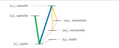
Figure 1. The energy diagram of the desired atom in our general protocol. The line width corresponds to the transition strength. The line colors indicate the relative energies of the transitions e.g. the blue line has a higher frequency than the green line.
