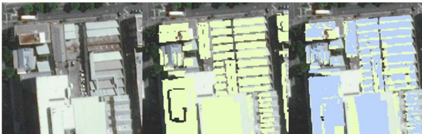
Example of good agreement between the two input data sources for large buildings. Aerial image (Left), AAM 3D buildings with Insolation limit method (centre); LiDAR with Insolation limit method (Right)
