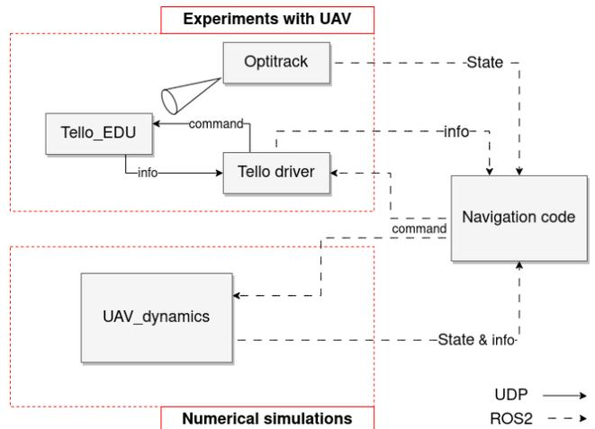
Fig. 4. System architecture. The upper red square shows the architecture used in the experiments with UAV, while the one in the bottom corresponds to the simulated dynamics. The different communications links are represented like displayed in the legend.
