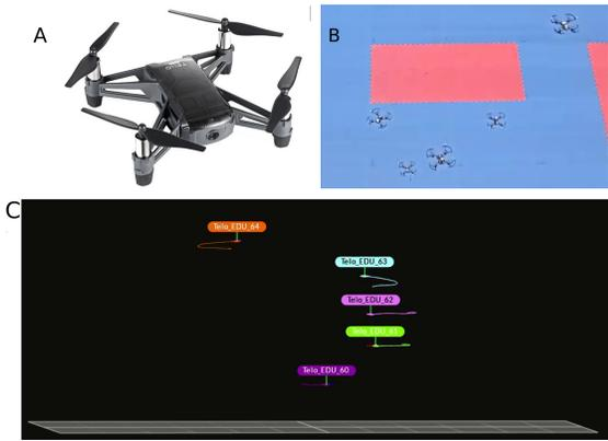
Fig. 3. [A] The experimental UAV, a Tello EDU<sup>®</sup><sup>3</sup>; [B] the view of the swarm within the flying arena (a 3-meter radius circle) and [C] A side view of the fleet through the motion capture tool used. UAVs fly in specific levels of altitude to avoid any collision, but are considered at the same height within the control algorithm
