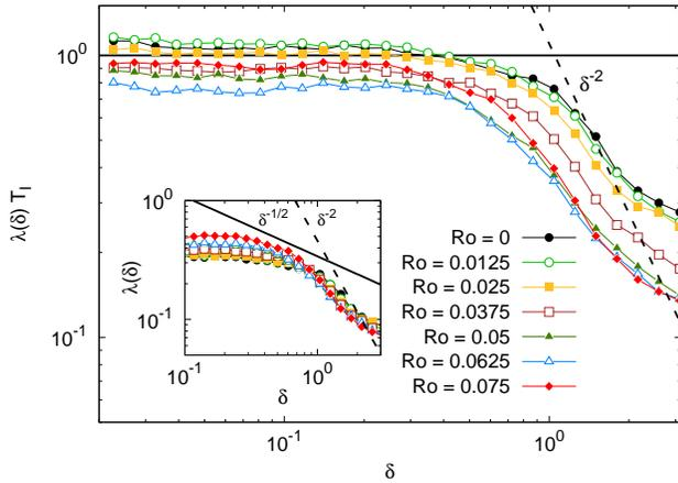
FIG. 4. FSLE (rescaled by the flow integral time scale) for different Rossby numbers. Inset: the same without rescaling the FSLE. The  $\delta^{-1/2}$  scaling law is the dimensional prediction for a kinetic energy spectrum  $E(k) \sim k^{-2}$ . The scale amplification factor is  $r = 1.2$ , and it was verified that the results are robust with respect to the choice of this parameter value.
