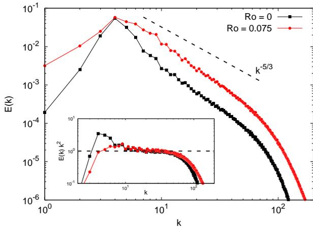
FIG. 1. Kinetic energy spectra, temporally averaged over several flow realizations in the statistically steady state for  $Ro = 0$  and  $Ro = 0.075$ . The dashed black line in the main panel corresponds to the expectation for SQG dynamics. Inset: the same spectra compensated by  $k^{-2}$  and rescaled with a coefficient such that, in both cases, the scaling range corresponds to the wavenumbers for which  $E(k)k^2 \simeq 1$ .
