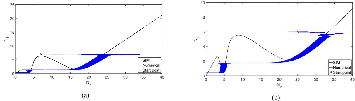
Figure 3: SIM and corresponding numerical free responses: a) System with the nonlinearity of Fig. 2a and initial conditions  $(w, v, \dot{w}, \dot{v}) = (7, 7, 0, 0)$ ; a) System with the nonlinearity of Fig. 2b and initial conditions  $(w, v, \dot{w}, \dot{v}) = (6, 25, 0, 0)$ .
