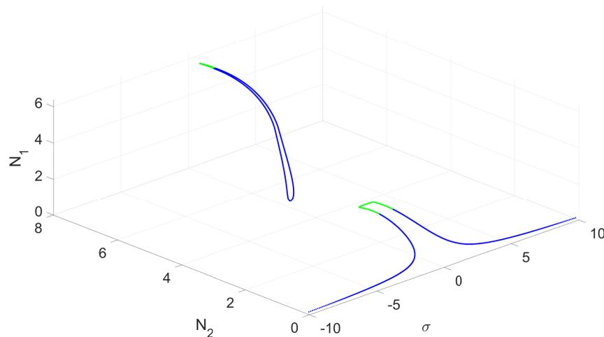
Figure 4: Detected equilibrium points of the system with respect to the de-tuning parameter  $\sigma$  for the system with restoring forcing function of Fig. 2a.  $\sigma$  is a de-tuning parameter representing a sweep of the frequency of excitation around the frequency of the outer mass (the system is studied around a 1 : 1 resonance).
