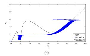
Figure 3: SIM and corresponding numerical free responses: a) System with the nonlinearity of Fig. 2a and initial conditions  $(w,v,\dot{w},\dot{v})=(7,7,0,0)$ ; a) System with the nonlinearity of Fig. 2b and initial conditions  $(w,v,\dot{w},\dot{v})=(6,25,0,0)$ .
