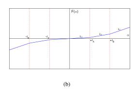
Figure 2: Considered nonlinearities for the restoring force  $F(\alpha)$ : a) Pure cubic and linear; b) Piece-wise linear.
