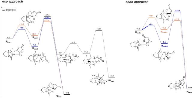
Figure 3. Computed exo- and endo- pathways. Z=C(CO<sub>2</sub>Me)<sub>2</sub>, [Co]=CpCo. ΔG are computed at the TPSS-D3/def2-TZVP level (T=383.15K). Solvent effects are added as single point calculations with the COSMO implicit model (toluene).
