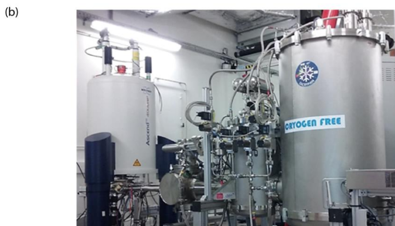
171 172 Figure 1. (a) Schematic of the closed-loop helium spinning system built at CEA Grenoble (b) Corresponding 173 photograph of the system, the probe being in the NMR magnet bore.
