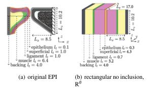
**Figure 1**. Silicone VF replicas without inclusion (dimensions in mm): a) molded EPI VF replica (right VF) and its schematic four layer anatomic representation, b) derived rectangular four layer replica ( $\mathbb{R}^{\emptyset}$ ).
