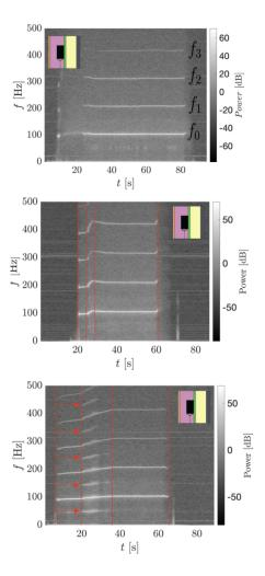
**Figure 4**. Upstream pressure spectrograms measured for rectangular replica with serial inclusion.
