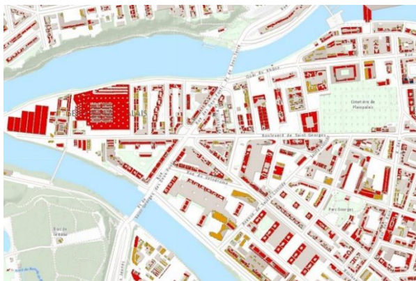
Figure 1: Solar irradiance as displayed by the solar cadastre of Geneva. Orange colour indicates a roof that receive between 1000 and 1200 kWh/m 2 /y. Red colour indicates roofs that receive more than 1200kWh/m 2 /y
