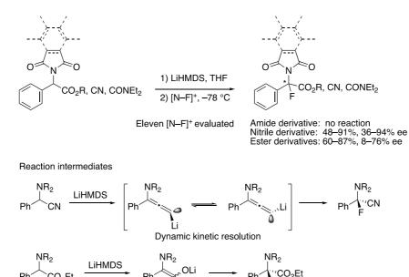
Facial differentiation **Scheme 4.** Enantioselective electrophilic fluorination of *N*-protected phenylglycine derivatives using various [N–F]<sup>+</sup> *Cinchona* alkaloids.
