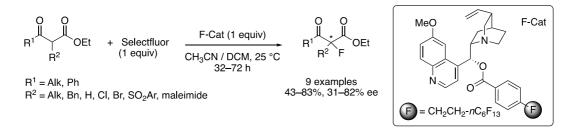
Scheme 20. Fluorination of β-ketoesters with Selectfluor / Fluorous CA.
