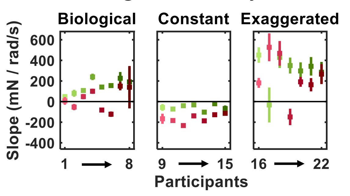
Magnitude of applied force correlated with the robot's angular velocity (H3 supported).
