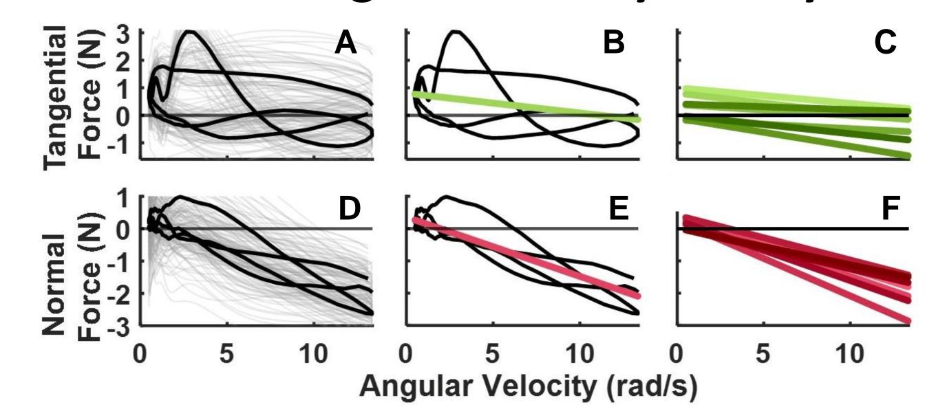
Slopes of linear regressions quantified how applied forces depended on the robot's angular velocity. Figures above show tangential and normal forces of the *constant* velocity profile.
