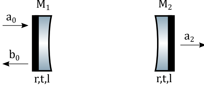
FIG. 11. Schematic of a 2 mirror cavity. a_0 represents the incident optical field at the input side of the cavity, assumed to be perfectly coupled to the cavity fundamental mode. b_0 represents the reflected optical field at the input of the two-mirror cavity. The parameter a_2 represents the optical field transmitted through the cavity. Parameters r, t, l represent the reflection, transmission and losses coefficients of the cavity mirrors.
