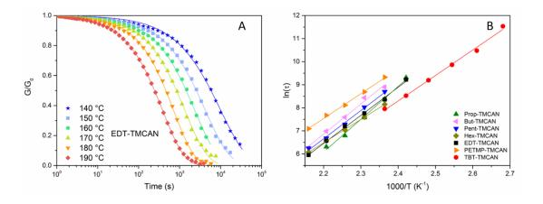
Figure 4. A) Normalized stress relaxations for EDT-TMCAN and B) Arrhenius plot of TMCANs.
